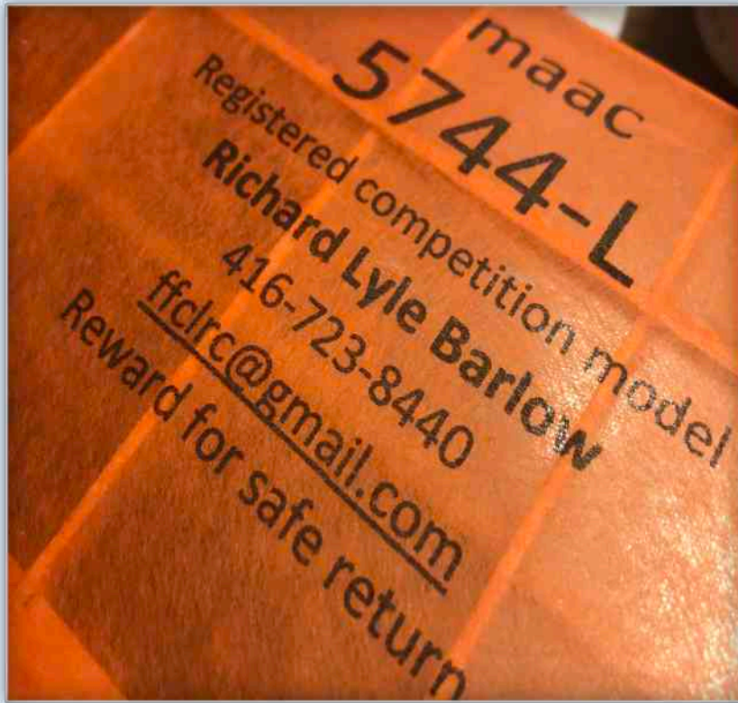
Above: Address labels Tape the jap tissue on the forward edge only to avoid jamming in the printer. Spray the dope, because if brushed, the lettering can dissolve and smear.
